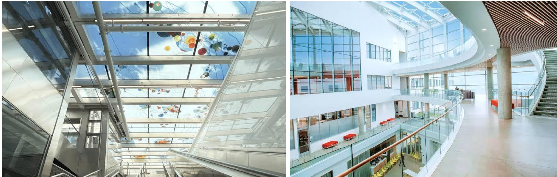
Figure 2.2: Atrium for Daylighting
